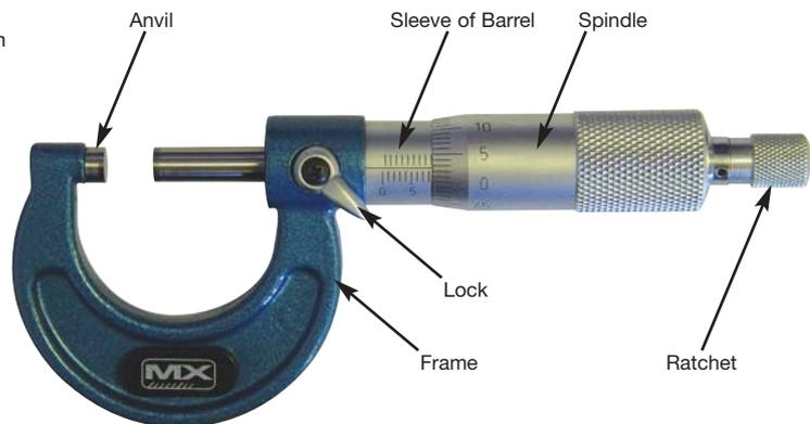
To get to the final reading size of a micrometer above we add up the three readings
